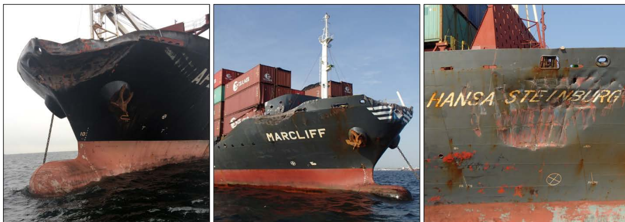
Damage to APL Guam bow (left); Marcliff bow, starboard side, and container (center); and Hansa Steinburg starboard-side bow. (Source: US Coast Guard)
